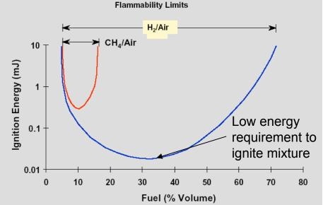
The range of flammability of  $H_2$ /air mixtures is wide. However the lower limit, which is normally most important (i.e. the point at which the mixture first becomes flammable) is similar to that of a methane/air mixture.
