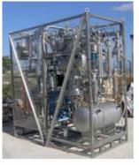
25kW electrolyser at the CRES facility
