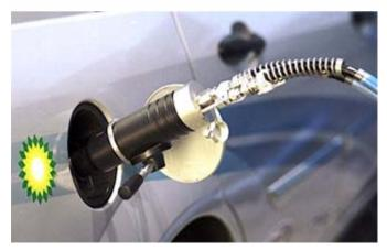
Connection of a hydrogen dispenser nozzle for filling with compressed hydrogen Images: Ludwig-Bolkow-Systemtechnik
