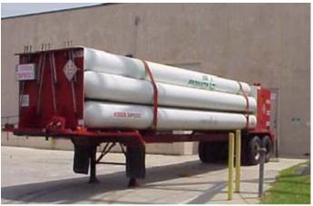
(Above) Hydrogen tube trailer containing approximately 300kgH<sub>2</sub>. Source: Air Products
